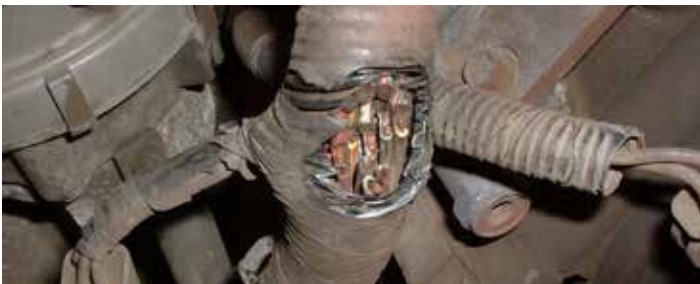
Sometimes the trouble is obvious. This harness was rubbing against the serp.
