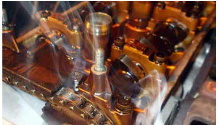
Injecting smoke into the spark plug hole is what found the bad piston.]
