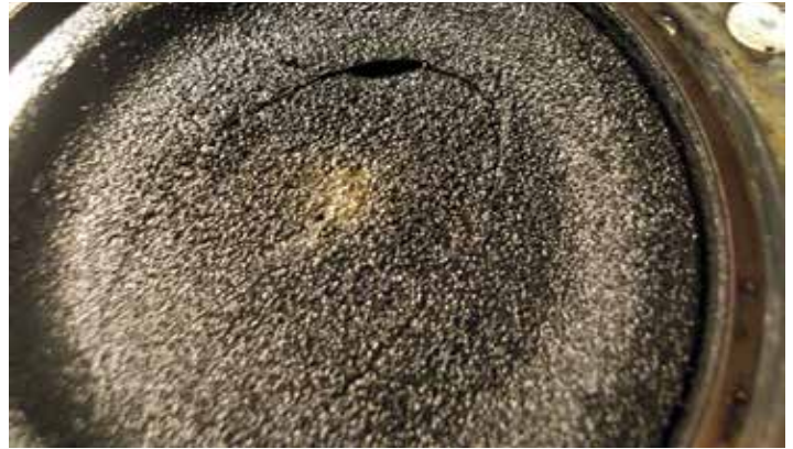
OBD II gave us the P0300 code for "random misfire" when a hole in the piston was the cause of the problem.
