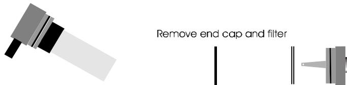
Remove the end cap from the in-line filter housing. Carefully remove the paper filter element and dispose of it. Clean the inside of the filter housing with a suitable soft cloth. Insert a new filter element onto the spigot in the filter housing and carefully replace the end cap.
