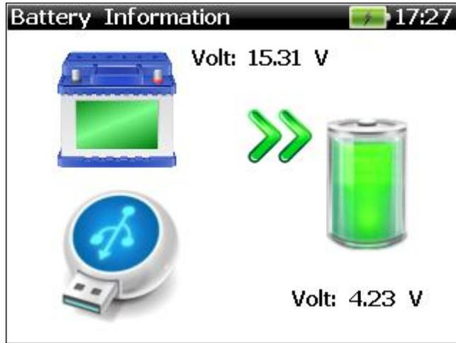
When the device is connected to the PC or to the external power supply, the power source comes from the USB interface and the battery screen changes as follows:
