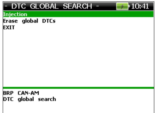
Proceedures to the errors reading as the chapter “READING STORED FAULTS”. Select “Erasing global DTCs” and the following confirmation message appears:
