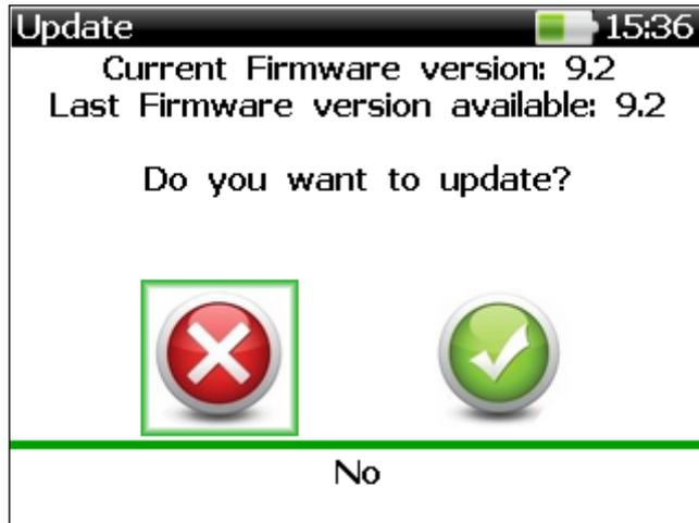
When a new software release is manually loaded into the device SD memory, to update the internal firmware, answer YES to the update confirmation message and wait until the procedure is successfully completed. Answer NO if you do not wish to proceed with the update.
