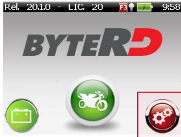
Select the SETUP icon (gears logo) using the left and right arrow keys and confirm with ENTER. The menu shown below appears on the scan tool:
